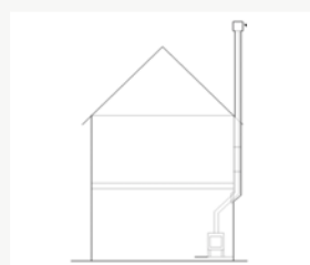
7. External wall penetration
