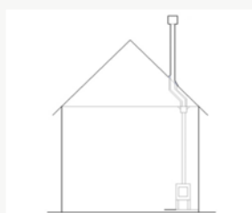
5. Flat ceiling with roof space and offset
